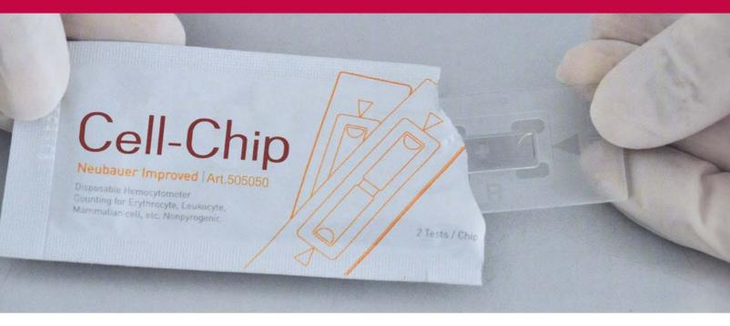
The counting chamber looks like the familiar Neubauer "improved" hemocytometer: The cells are distributed over  $3 \times 3$  large squares, each with 1 mm edge length and with a surface area of  $1 \text{ mm}^2$ .
